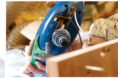
The rower is driven by an 'O' ring tensioned by a jockey wheel. The thin white tube is the cable that operates his jaw
