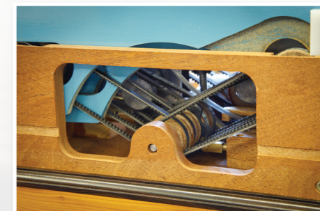
View of the interior, showing some of the 17 German-built cam belts and pulleys. Matched pairs of pulleys, all at slightly different diameter changing the ratio of the wave cams, produce a random pattern of movement
