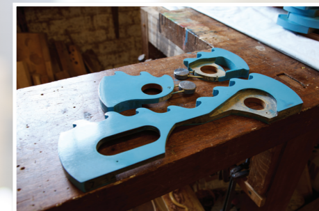
Full wave and pair of half waves showing slot to accommodate an eccentric cam, allowing for movement
